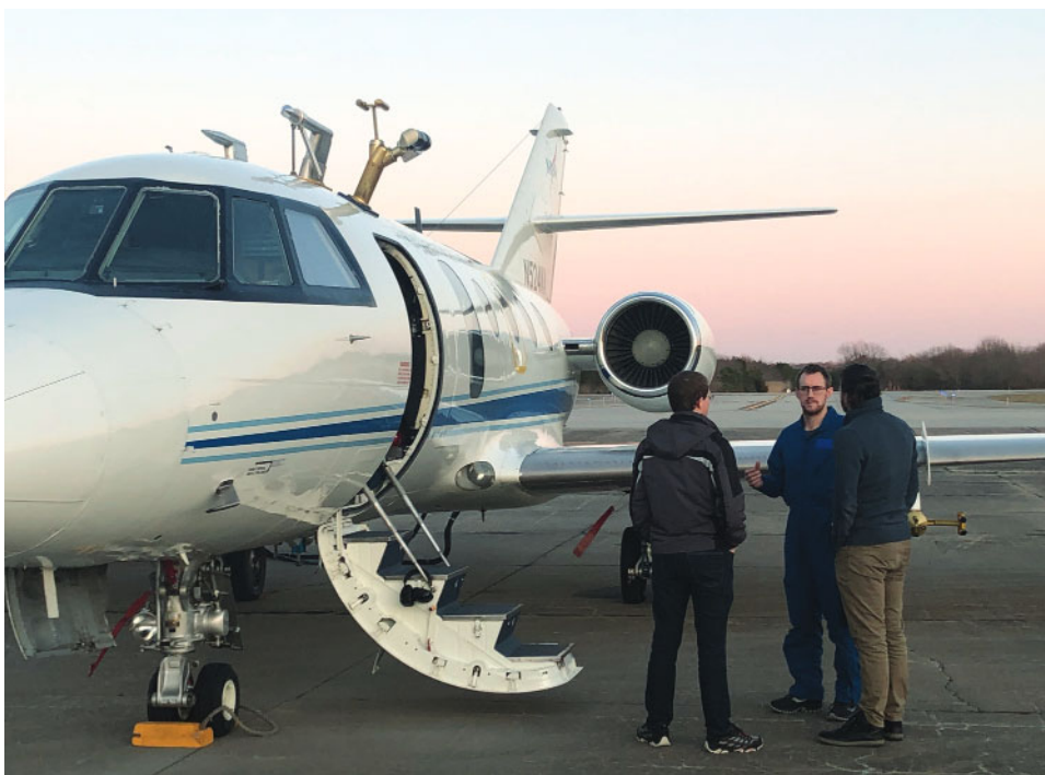
Figure 5. ACTIVATE scientists Ewan Crosbie (facing camera) talking to Michael Shook and Simon Kirschler after an ACTIVATE flight. Note the sampling probes on the top of the aircraft. Photo credit: Armin Sorooshian
